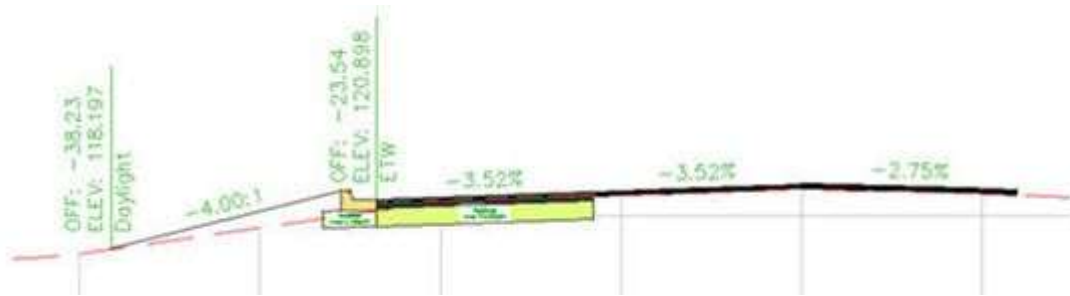
Figure 44: Same section view using a customized code set style. Note the labels, as well as the differentiation between materials.
